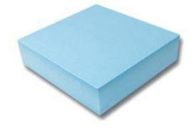
**STYROFOAM™** Brand HIGHLOAD 60 Insulation has a minimum compressive strength of 60 psi (415 kPa). The Type VII extruded polystyrene foam insulation resists compressive creep and fatigue, delivering long-term compressive strength and thermal performance in high-load applications.
