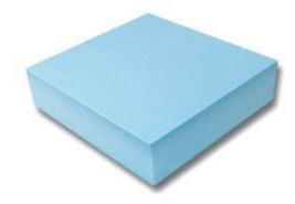
**STYROFOAM™ Brand HIGHLOAD 100** Insulation has a minimum compressive strength of 100 psi (690 kPa). The Type V extruded polystyrene foam insulation resists compressive creep and fatigue, delivering long-term compressive strength and thermal performance in high-load applications.
