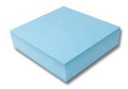
STYROFOAM™ Brand DECKMATE™ Plus Insulation is a Type IV extruded polystyrene foam product designed for use on conventional roofs beneath mechanically fastened, fully adhered or ballasted sheet membranes. It can be used on built-up, modified bituminous and metal roofs, and installed directly on a steel deck without the use of a thermal barrier such as gypsum board.
