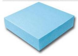
**STYROFOAM™** Brand HIGHLOAD 40 Insulation has a minimum compressive strength of 40 psi (275 kPa). The Type VI extruded polystyrene foam insulation resists compressive creep and fatigue, delivering long-term compressive strength and thermal performance in high-load applications.
