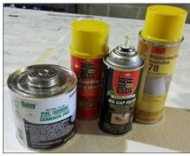
PVC Cement was used to make the mortar joints. You may want to practice on some scrap material to develop your technique. We also did various tests with the adhesives to see how they performed; bond strength, drying time, surface preparation, etc.
