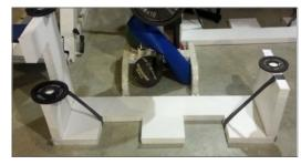
We made use of duct tape and weights from our home gym to apply pressure to joints to ensure a good bond.
