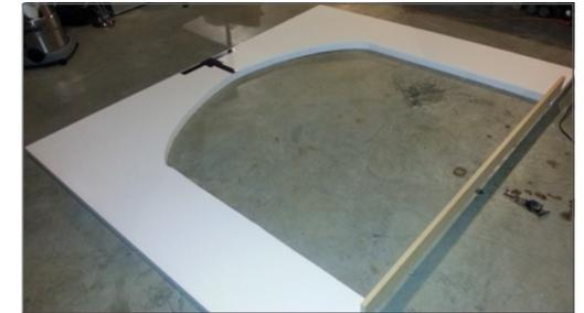
Our castle was built in four sections. Each section was reinforced with a wood frame made from 2x4s and 1x4s across the bottom of the openings. The wood was bonded to the foam using Loctite Foamboard Adhesive available from Home Depot.
