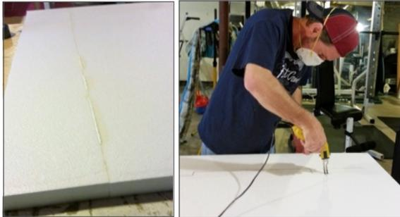
We use a hot knife foam cutter from Demand Products. The sheets are cut and then bonded together with 3M #78 if the fit is perfect (finished edge to finished edge) where a cut edge is bonded, Great Stuff fills the gaps and sets up like a rock. A large T Square works well to lay out the grid for the mortar joints.
