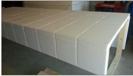
The wooden frames on the towers worked as a stand to do the painting and mortar joint work. Once on the stage, the top frame was removed and the tower stood on the bottom support.
